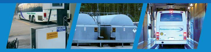
The detectors for cardless refuelling are contained inside the fuel dispenser nozzle (black collar) and in the fuel tanks of the buses. Information about the fill-ups is sent automatically to the LabkoNet® system. This way, the level control automatics will know that the amount of fuel in the tank is not decreasing because of a leak.
